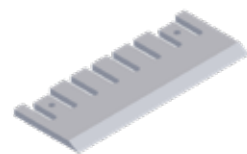
HOGGING KNIFE 765 × 295 × 25 mm 8 notches, 2 recesses in spine, 2 M12 threads in spine
