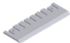
HOGGING KNIFE 870 × 295 × 25 mm 9 notches, 2 recesses in spine, 2 M10 threads in spine
