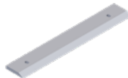
HOGGING KNIFE 530 × 85 × 14 mm 2 M8 threads in spine
